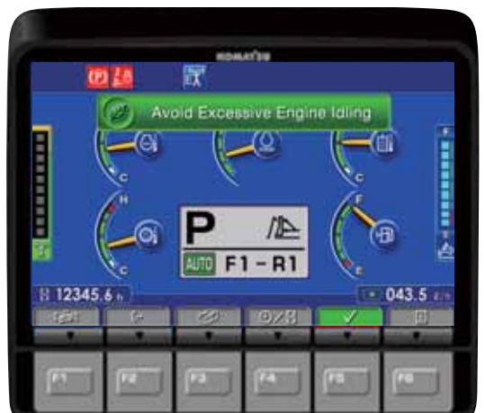
Eco gauge, eco guidance and fuel consumption gauge help to further reduce consumption.
