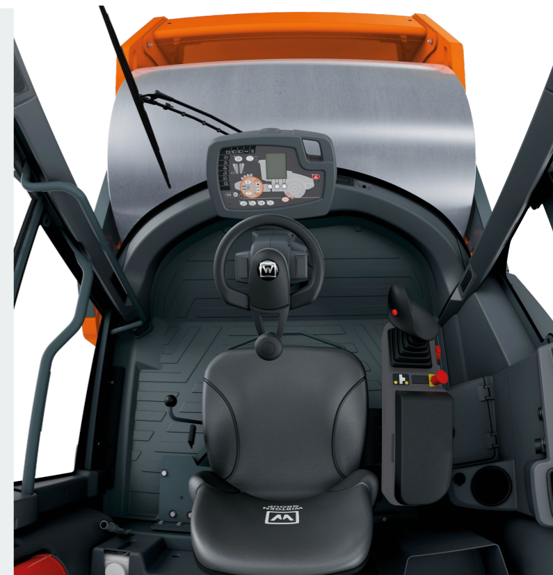
The important buttons are visible at all times in the spacious Easy Drive operator's platform. The idea behind all other operating elements is that, the more often they are used, the closer to the joystick they are located.
