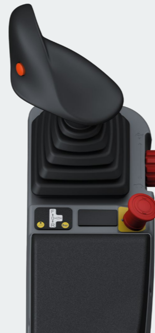
Drive control is by means of a joystick on the multifunction armrest.
