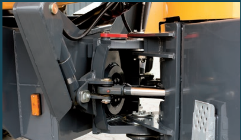
Articulated swivel joint with stabilization cylinder.
