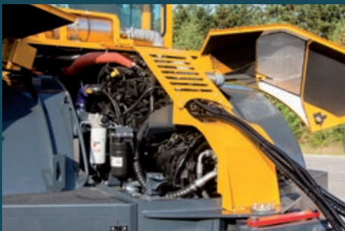
Good access to all maintenance points with the patented hood system.
